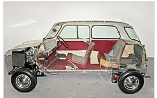
A cross-section shows how a Mini maximises passenger space.
