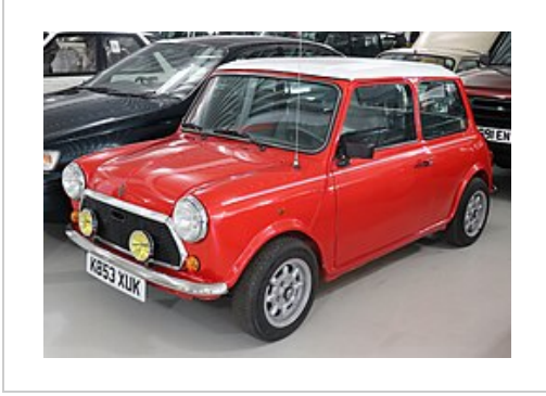
1992 Mini Cord built with a fibreglass body
